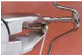
14 Activation: Remove security thread
