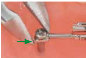
19 Slide the c-clip off the screw
