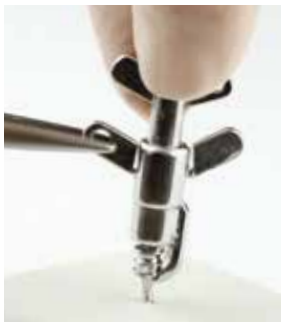
Attachment of the collar extractor
