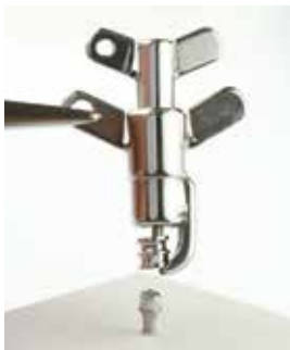
Removed collar in the collar extractor
